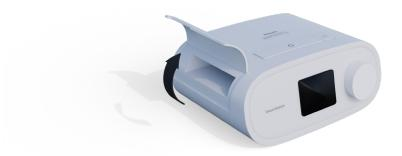
2. Remove the modem accessory door from your DreamStation device by lifting and firmly sliding the door to the left and pulling the right side of the door toward you until it pops out. This may take several attempts.
